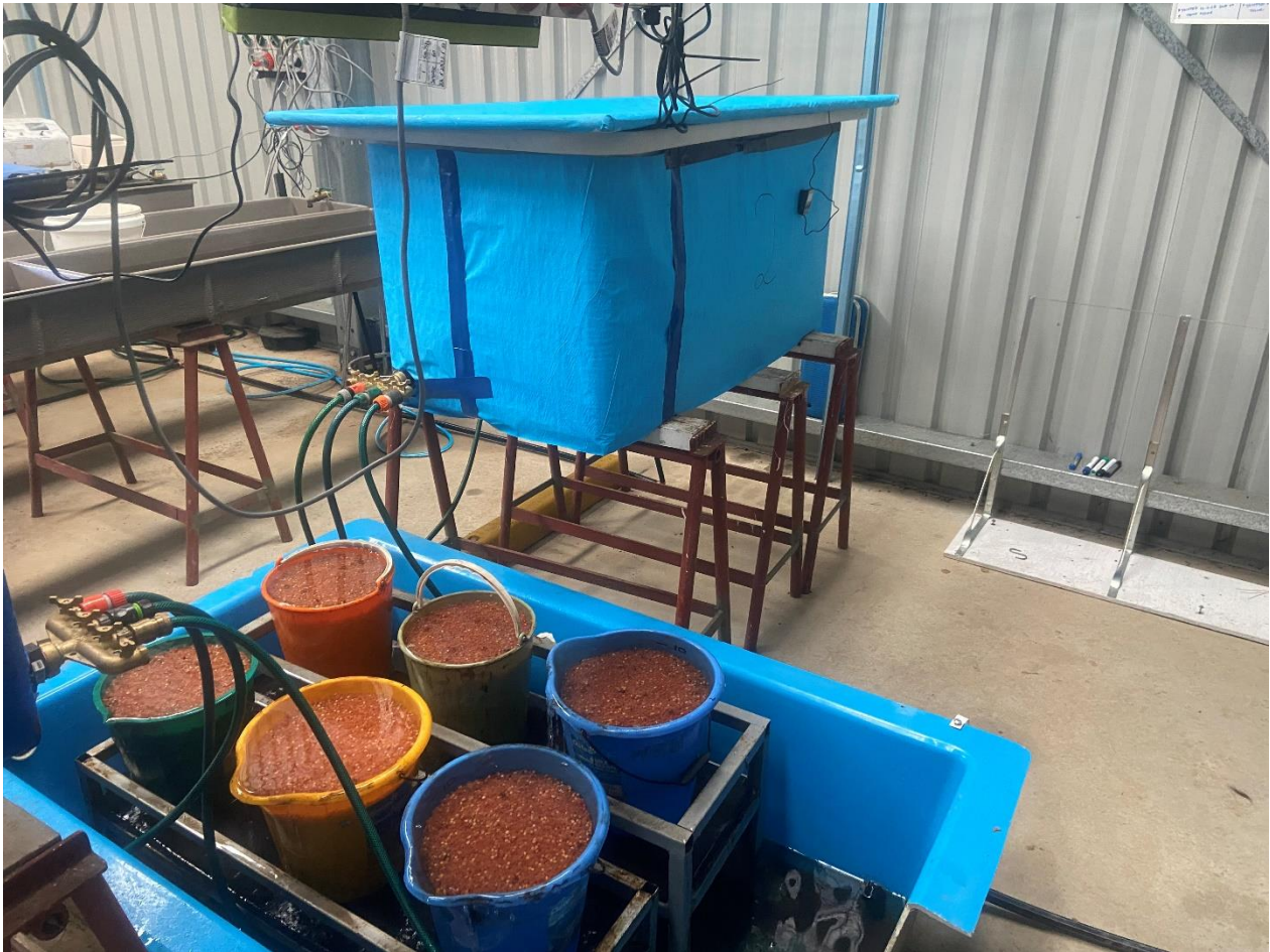
Egg Upweller system designed to heat up the water to 10 degrees Celsius, the optimum growth temperature for salmonids
